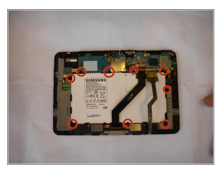
Use a Phillips #00 screwdriver to remove the nine 1 mm screws located around the battery.
