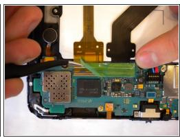
• Use tweezers to peel up the green tape located on top of the two flexible ribbon cables.
