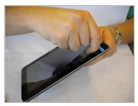
Insert a plastic opening tool between the back cover and the screen of the Samsung Galaxy Tab 8.9.
