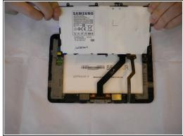
• Use a spudger to lift up and separate the battery from its housing.
