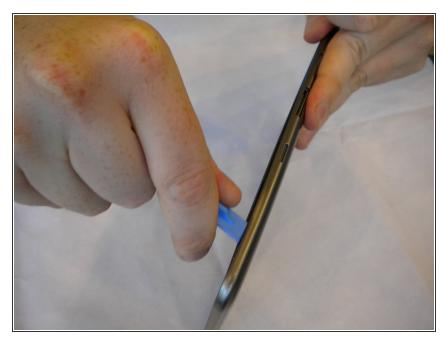
Slide the second plastic opening tool along the edge of the device to separate the back cover from the screen.
