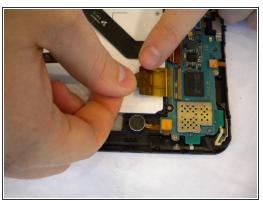
Carefully pull out the yellow flexible ribbon cable to disconnect it from the motherboard.
