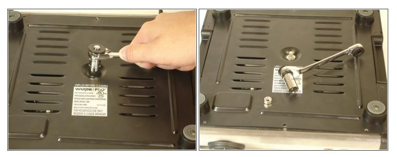
Using a wrench, remove the bolt from the center of the back panel.
