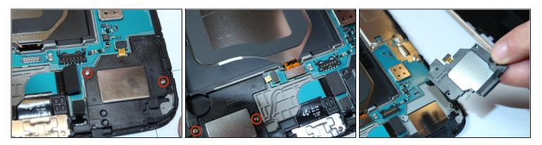
• Unscrew the 2.9mm screws from the speakers using a Phillips head #000 screwdriver, then lift the speakers from the device.
