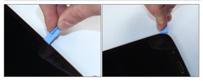
• Start out by separating the screen from the back cover using the larger plastic opening tool to pry them apart.
