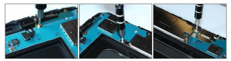
• Unscrew the one 2.9mm Phillips #000 screw above the battery, and the three 2.9mm Phillips #000 screws to the right of the battery.
