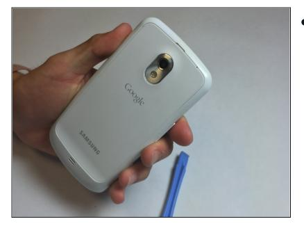
• You must open the back of the phone to access the battery. To do this use the plastic opening tools or your fingernail and insert it into the divot.
