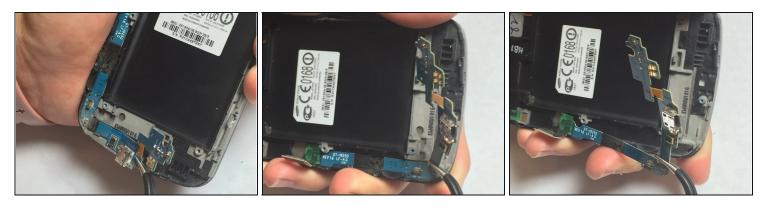
• With your <u>tweezers</u> remove the bottom circuit from the screen.
