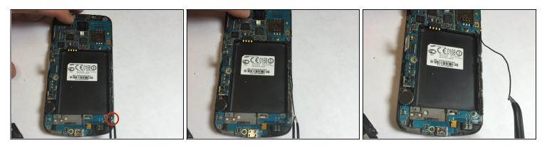
• Remove the antenna using either your fingers or tweezers.
