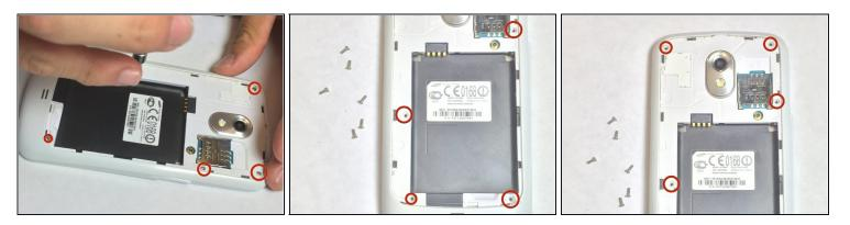
• Remove 4.4 mm screws using a PH # 000 as indicated on the picture.
