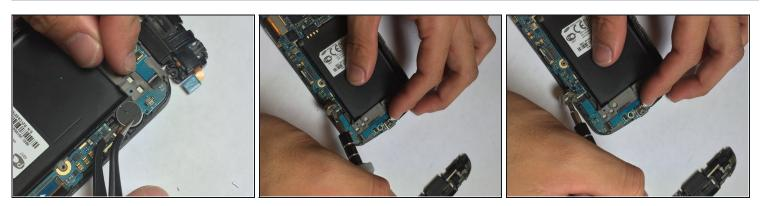
• Remove the internal battery using <u>tweezers</u> or your flat head screw driver.
