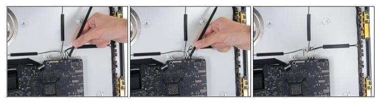
• Use the flat end of a spudger to disconnect each of the four antenna connectors from the AirPort/Bluetooth card.
