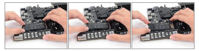
$\triangle$  To avoid damaging its socket, do not lift the end of the SSD above about 15°.
