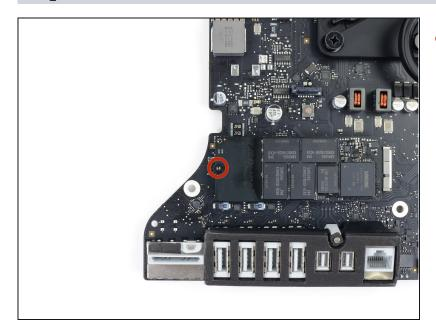
Remove the single 5.3 mm T8 screw securing the SSD to the logic board.
