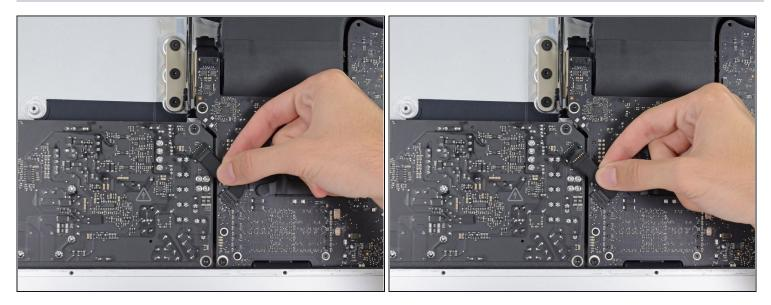
A When working on the power supply, **be very careful** not to touch the capacitor leads or any exposed solder joints on the back of the power supply. Only handle the board by the edges.
