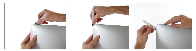
• Push the tool around the top right corner of the display.
