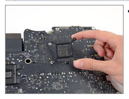
• Remove the bracket from behind the GPU heat sink.
