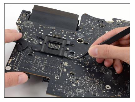
• Remove four black stickers from the back of the CPU heat sink.
