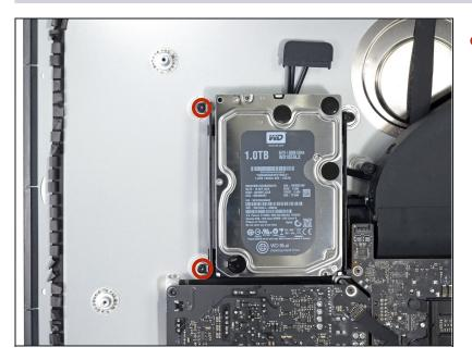
Remove two 7.3 mm T10 screws securing the left hard drive bracket to the rear case.
