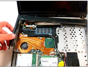
• Starting from the bottom right, carefully pry off the bezel. Use a spudger or flathead screwdriver if assistance is needed.
