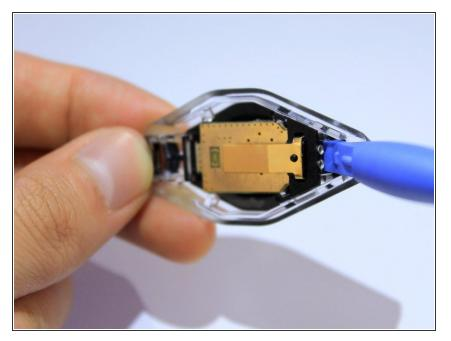
Place the plastic opening tool behind the logic board and bend away from the casing
