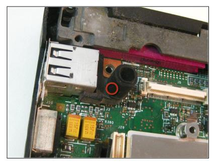
Remove the rubber cover from the microphone.
