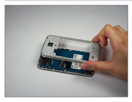
Carefully separate the rear housing and the mid-frame to reveal the inside of the phone.
