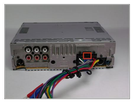
Locate the clip on the wiring harness.
