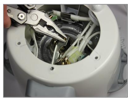
If the brass beam can't fit through the hole in the silvercolored beam, use pliers to bend the brass beam outwards so that it does not fit through the hole in the silver-colored beam.
