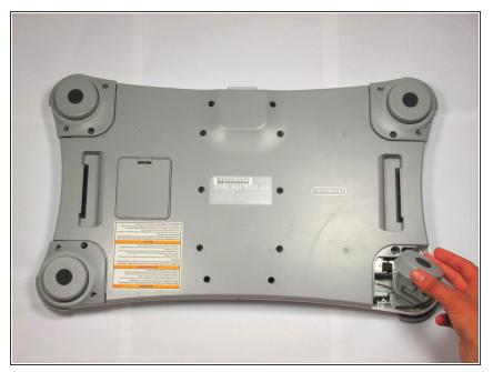
Separate the loose foot from the device by lifting it up.
