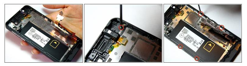
$\bigwedge$  The screen is fragile and may crack if the screws are not removed carefully.
