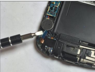
With the flat head screw driver pull up the blue connector.
