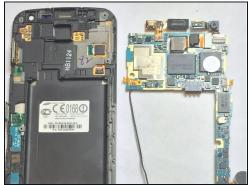
• Using tweezers, pull the top circuit board off.
