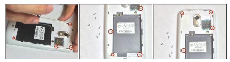
• Remove 4.4 mm screws using a PH # 000 as indicated on the picture.
