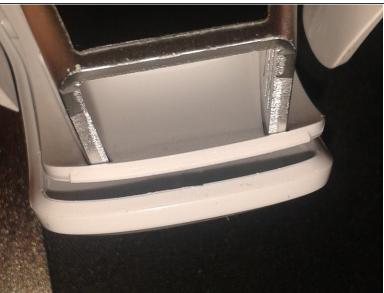
↑ BE CAREFUL WITH FLAT-HEAD SCREWDRIVER! Alternatively open it bare handed.
