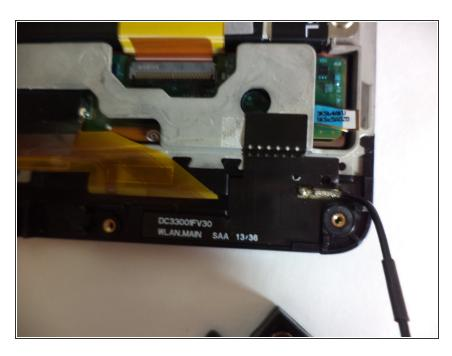
Detach the Wi-Fi antenna transceiver from the display panel assembly that is attached with adhesive.
