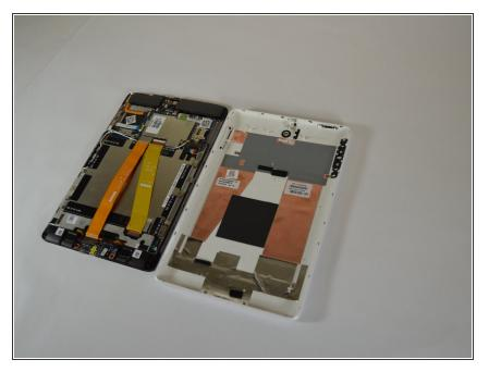
• Use plastic tool to remove the back cover.
