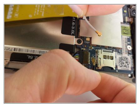
• Release the Wi-Fi antenna cable from the routing clips and channel from the main board.
