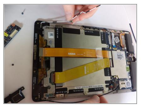
• Detach the Wi-Fi antenna from the main board.
