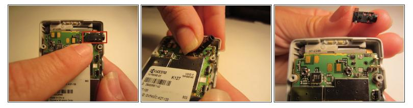
Locate the headphone jack attached to the top right of the motherboard and pull it off using your thumb and index fingers.
