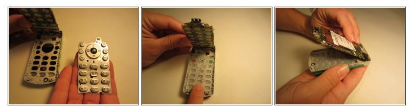
• Hold the new keyboard in your hand facing you as it would look in your cell phone, lift the motherboard with your opposite hand, and then flip the keyboard face down and fit it in to place.
