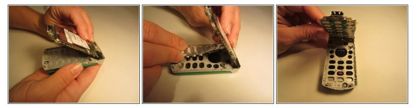
• Lift the motherboard away from you to locate the existing keyboard and remove it.
