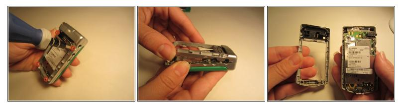
Use the Y1 tri-wing screwdriver to remove the four 2.4mm screws and then pry the entire backing
