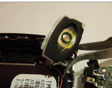
Once the two screws that hold the speaker in place are removed, remove the speaker using tweezers.
