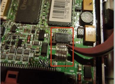
In order to get to the speaker, try to free the motherboard by removing all the wires from their combs using the tweezers.
