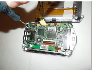
Once the backboard is removed, remove the four screws on the motherboard. Two on top of the motherboard and two on the bottom of the motherboard using the Phillips screwdriver.
