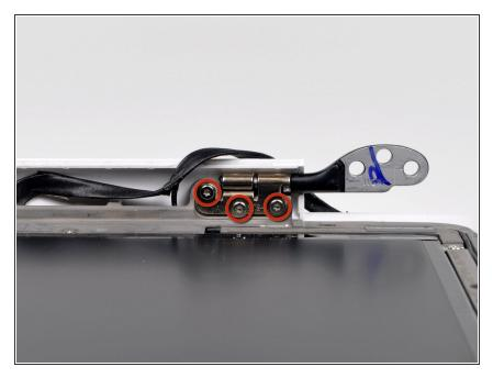
Remove the three 4.7 mm T6 Torx screws securing the left clutch hinge to the front display bezel.
