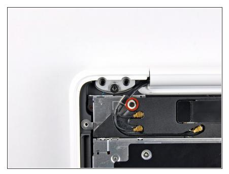
Remove the single 3 mm Phillips screw securing the AirPort/Bluetooth antenna ground strap to the rear speaker.
