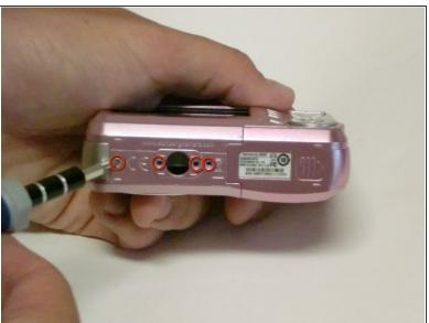
Remove all screws along the edges of the camera, using a #00 Phillips screwdriver.
