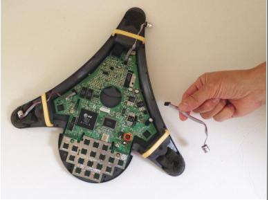
Gently pull up on the black plastic tab connected to the motherboard to disconnect each microphone.
