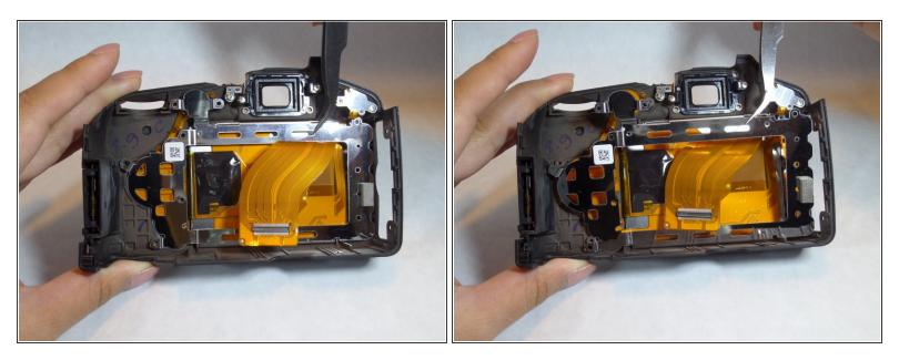
• Using a pair of tweezers, gently lift and remove the silver protector cover.
