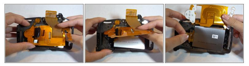
• Lift the yellow sheet to reveal the LCD screen.
