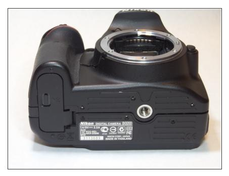
Locate the battery compartment on the bottom of the camera directly below the mode dial.
