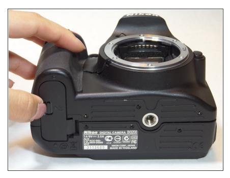
• Find the marked arrow on the battery compartment door and firmly push following the arrow's direction to release the latch.
