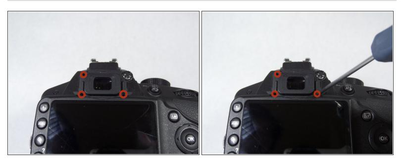
Locate and remove the 4 screws above the LCD screen, around the eyepiece. Use a razor to carefully peel the sticker off the +/- wheel to reveal the screw beneath.
