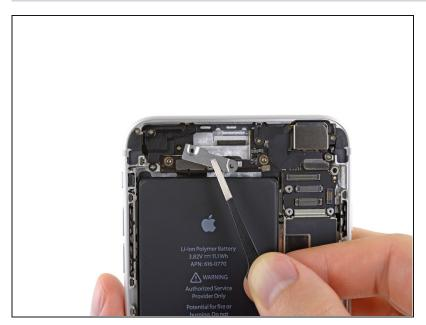
Grasp the 5GHz Wi-Fi antenna bracket with a pair of tweezers and lift it off the iPhone.
