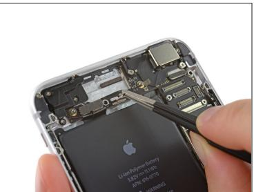
• Grasp the 5GHz Wi-Fi antenna connector with a pair of tweezers and gently lift it from its retaining clip on the logic board.
