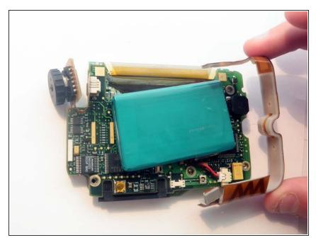
The conductor can now be easily removed by pulling it off of the logic board.
