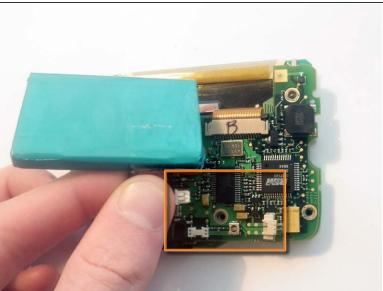
Gently pull on the wires connecting the battery to the device until the battery disconnects.
