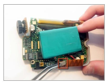
Disconnect the power conductor by gently peeling the grey section (which is connected to the logic board) upwards.
