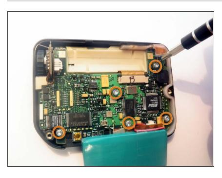
Use the T9 Screwdriver to remove the five visible screws: Top right, bottom right, middle center, bottom center, bottom left.
