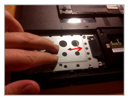
slip the case to the right to plug in the HDD/SDD again
