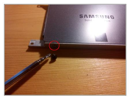
put the new hard drive or SSD, respectively in the case and fix the screws again (the HDD/SDD will only fit in the case in one way)
