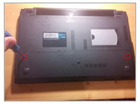
unscrew these two screws to remove the coverage
