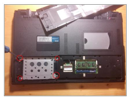
• unscrew these four screws to take out the case with the hard drive disk
