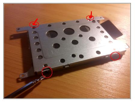
unscrew the four screws of the case to remove the hard drive out of that case
