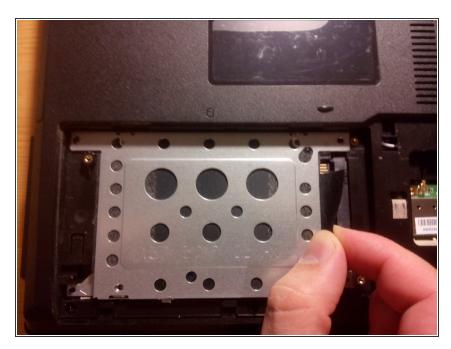
• pull the strap to remove the hard drive's case
