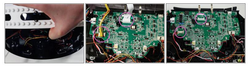
Detach the two circuit plugs connecting bObi's cover to the main board and the cover will be completely removed.
