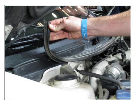
• Remove the rubber gasket from the rain tray.
