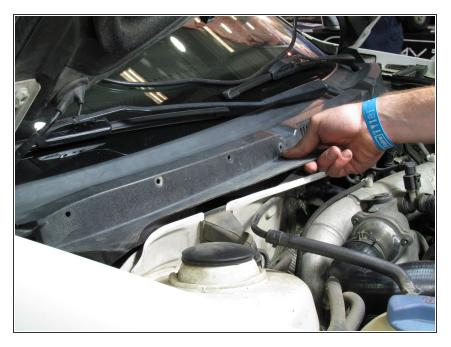
• Lift the tray upwards and away from the vehicle.
