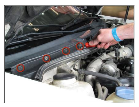
• Use a #2 Phillips screwdriver to remove the four screws.
