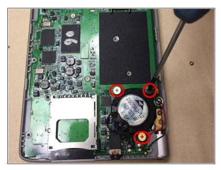
Remove the three silver screws from the black round battery using a Phillips #0 screwdriver.
