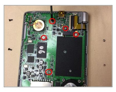
Remove the five small screws from the motherboard using a Phillips #0 screwdriver.
