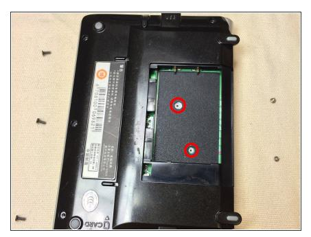
Remove the two screws behind the battery using a Phillips #0 screwdriver.
