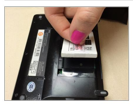
Pull upwards on the battery tab to remove the battery from the device.
