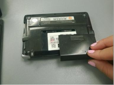
Place your fingers on the battery cover arrow and pull the cover down and off the device.
