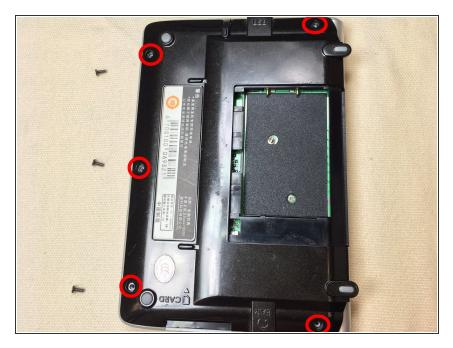
Remove the five screws around the edge of the device using a Phillips #0 screwdriver.
