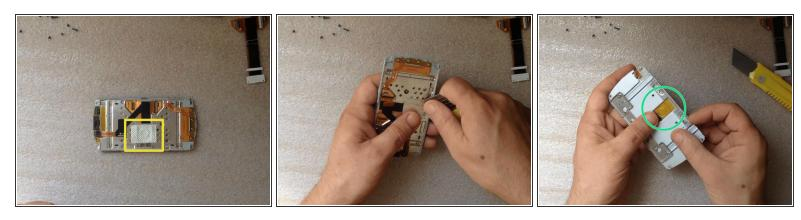
To release the ribbon cable peel off two patches.
