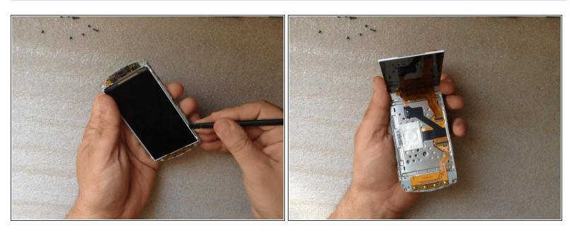
Use the thin end of a plastic tool to remove LCD Display and disconnect the flex cable.
