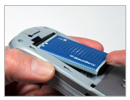
Remove the battery from the battery housing by flipping up the top of the battery.
