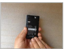
Switch-off the phone and remove the battery.
