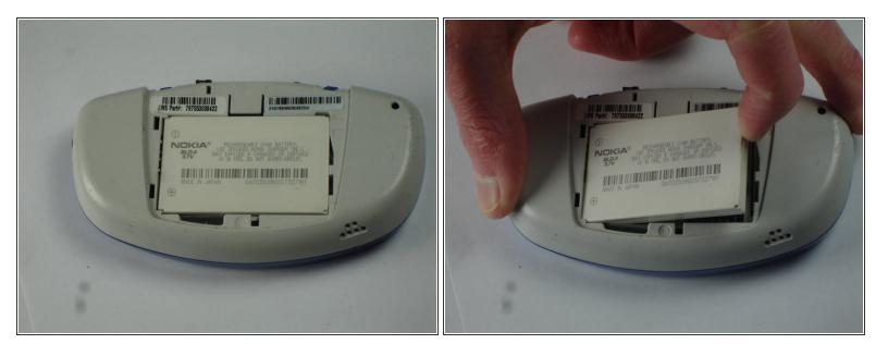
• Lift the battery out of the back of the phone.
