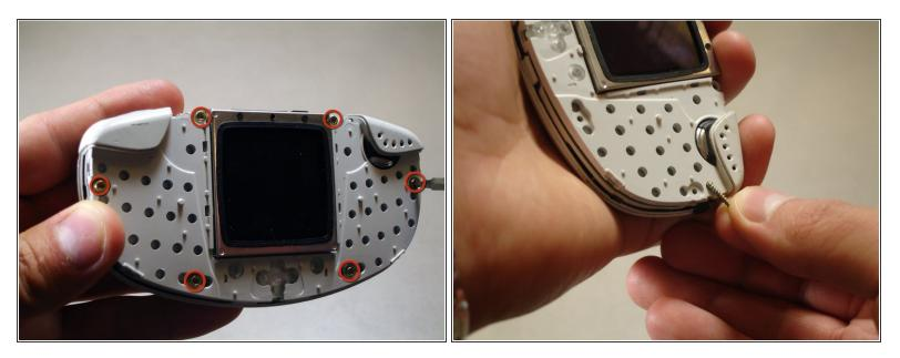
• Remove the six Torx T6 screws from the phone's front case.
