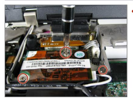
Remove the three screws holding down the modem in the upper left corner of the laptop.
