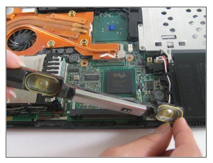
• Lift the speakers out by starting with the left end and then unsnake the wires.
