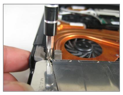
• Remove the screw on the left hand side of the case, above the expansion slot.
