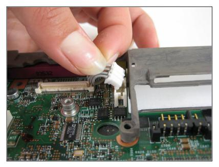
• Unplug the small ribbon cable attached to the motherboard.
