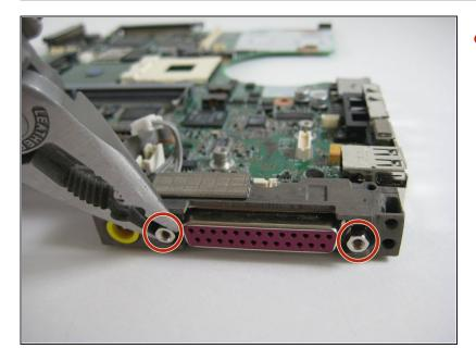
• Using a nut driver or a pair of thin nose pliers, remove the two stand off screws next to the pink parallel port on the back of the computer.
