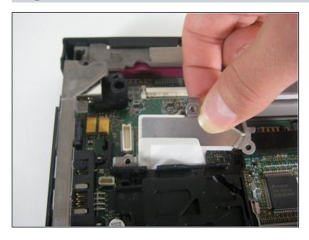
• Remove the sheet metal piece, which was underneath the modem.
