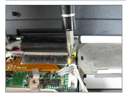
• Remove a single screw from the metal plate that secures the display cable.
