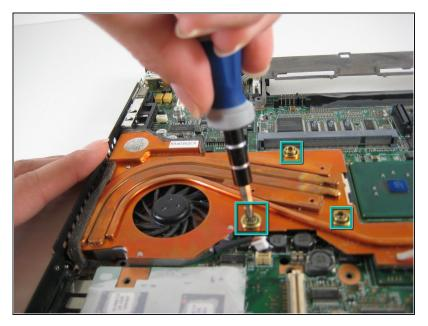
• Remove the three screws on the fan.
