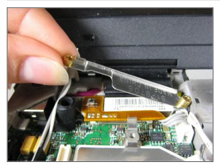
• Pull the metal plate away from the display cable.
