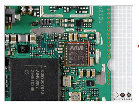
The <u>Wolfson Micro WM8903</u> is a low power stereo codec with all sorts of fancy features like programmable audio path control sequences, both pseudo-differential *and* fullydifferential analog inputs, a dynamic range controller, and all sorts of other technical jibber jabber.
