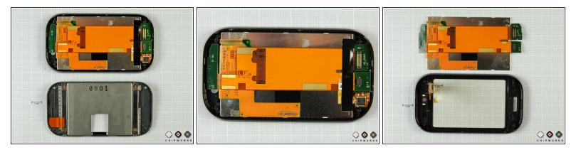
• Separating the two halves of the display assembly reveals a bunch of cables connecting the microphone, speaker, display, and digitizer to the main board.
