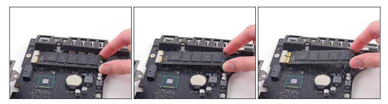
• Slightly lift the rightmost side of the SSD and firmly slide it straight away out of its socket on the logic board.
