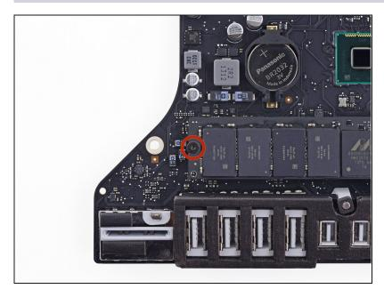
Remove the single Torx screw securing the SSD to the logic board.
