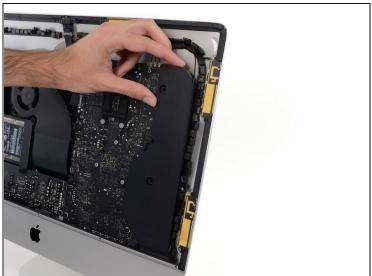
• Pull the top of the right speaker away from the rear enclosure, about half an inch, to expose the antenna cable running down its right side.
