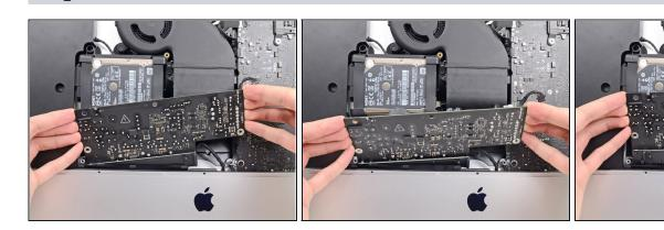
• Rock the power supply forward and remove it from its recess in the rear enclosure.
