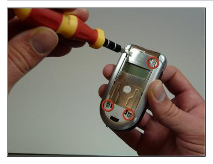
Remove the four screws securing the front cover.
