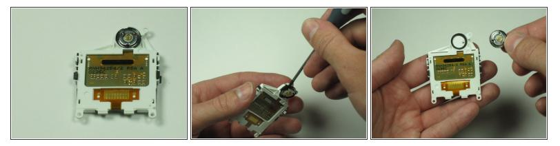
• Gently pry it out the speaker located in the screen housing with a small screwdriver or similar tool.
