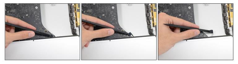
• Use the flat edge of a spudger to pry the headphone jack cable connector from its socket on the logic board.
