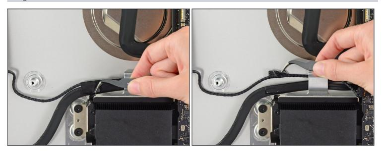
• If necessary, use a pair of tweezers to gently peel the tape securing the left speaker cable to the SATA data/power cable.
