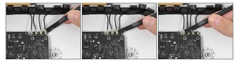
• Use the flat edge of a spudger to disconnect each of the four antenna connectors from the AirPort/Bluetooth card.
