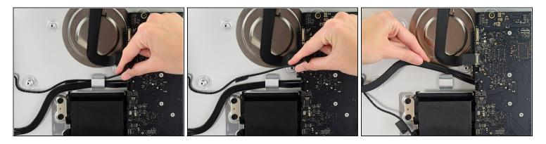
• De-route the left speaker cable by pulling it straight up out of the retaining clip in the back of the rear enclosure.
