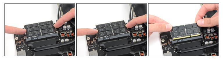
• Release the tabs on each side of the RAM module by simultaneously pushing each tab away.
