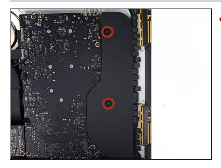
• Remove the two 10.0 mm T10 screws securing the right speaker to the rear enclosure.
