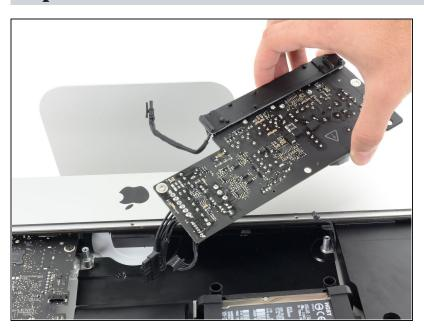
• Remove the power supply from the iMac.
