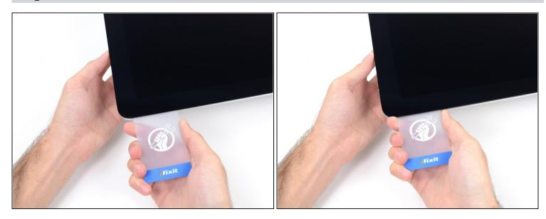
Wedge the plastic card into the top right corner once again, and leave it there to prevent the adhesive from resticking.
