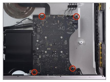
• Remove the four 7.2 mm T10 screws securing the logic board to the rear enclosure.
