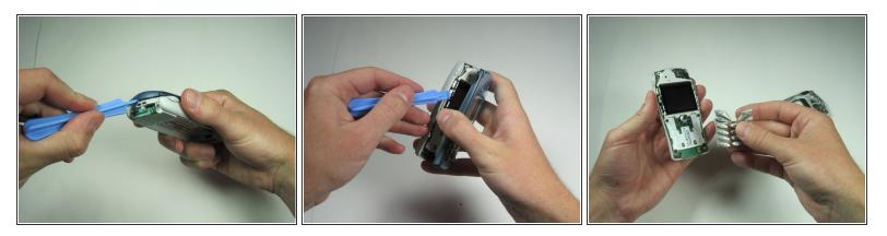
• After removing the screws, the two halves will separate. If not, then pry them gently apart.
