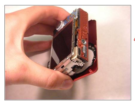
Gently loosen the front casing by gently using your fingers to pull it apart.
