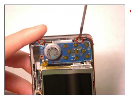
Remove the two screws at the top of the camera casing.
