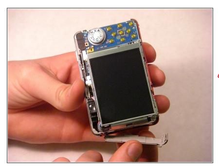
On the casing on the opposite side of the camera, gently loosen and remove the casing by firmly pulling with your fingers.
