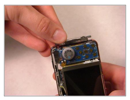
After removing the screws, gently pop open the plastic piece, as shown by firmly pulling it with your fingers.
