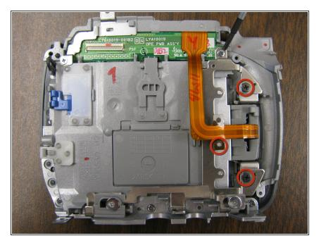
• Remove the 3 screws holding the LCD screen hinge to the base.
