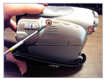
• Remove the 2 screws on the side opposite the LCD screen.
