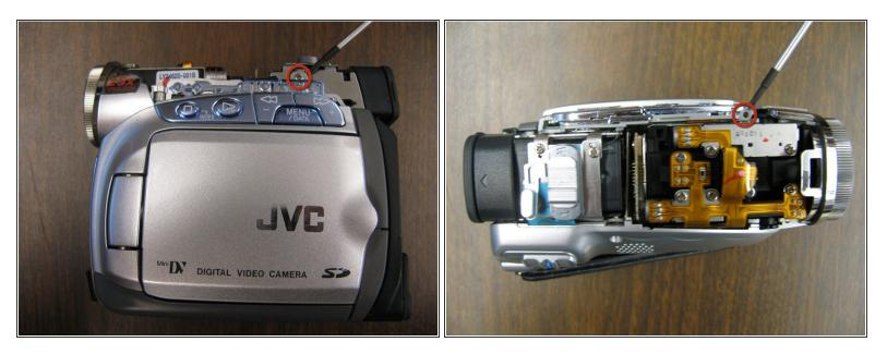
• Remove the 2 screws underneath the top cover on the LCD side of the camera.
