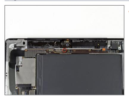
• Remove the single 2.6 mm Phillips #0 screw securing the camera cable to the headphone jack assembly.
