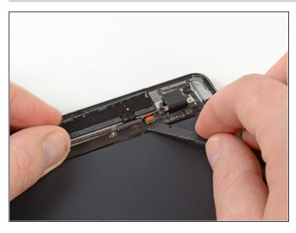
Use the flat end of the spudger to pry up the antenna connector cable out of its socket on the headphone jack assembly board.
