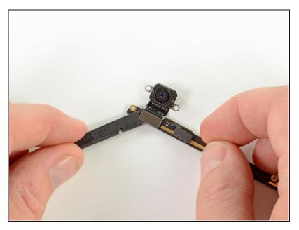
Using the flat end of a spudger, pry the rear facing camera off of its socket on the underside of the headphone jack assembly board.
