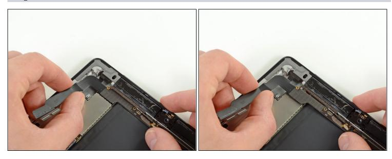
• Holding onto the ribbon cable of the headphone jack assembly, carefully pull the assembly parallel to the iPad, toward the bottom of the device.
