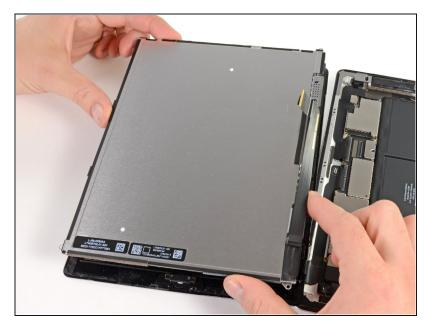
• Without touching the front of the LCD, lift the LCD off the front panel.
