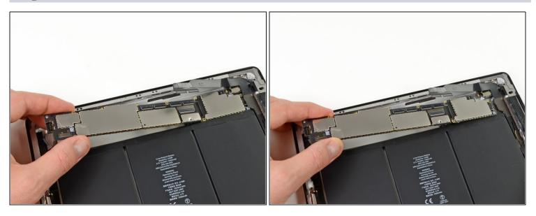
• Holding the logic board by the side nearest the dock connector, carefully pull the logic board toward the bottom of the iPad.
