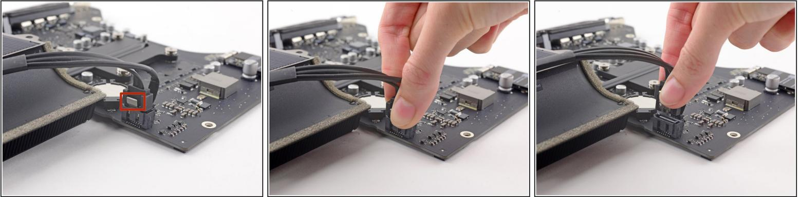
**i** The SATA data connector has a clip that must be pressed to allow removal.
