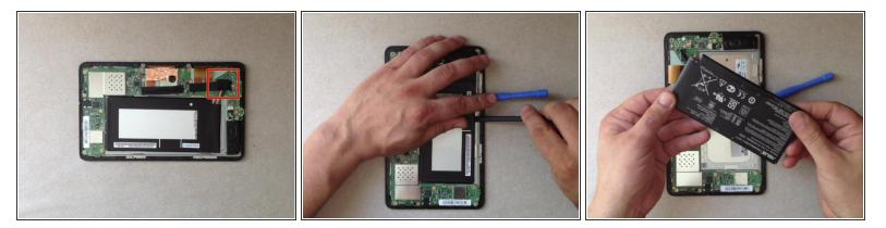
• Disconnect and remove the battery.
