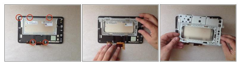
• Remove the metal LCD display shield.
